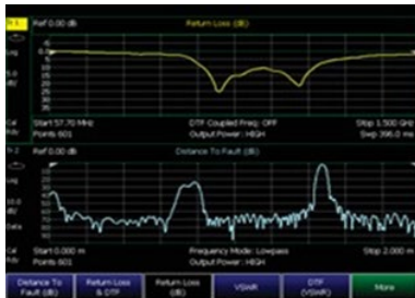
View return loss and DTF simultaneously
